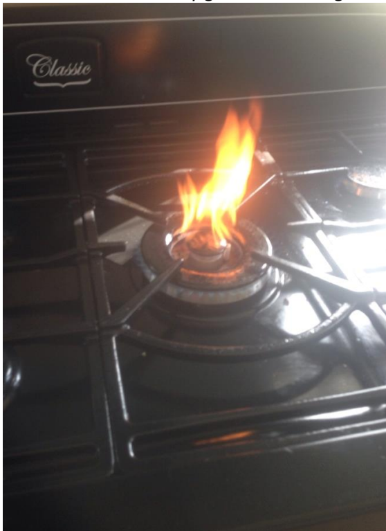
Photo 1. Bad flame picture and flame lifting from hob (Nat Gas set-up with LPG in use)
